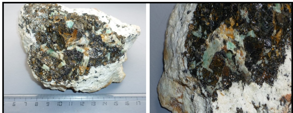
Figure 3 Left: Sample from the Novo Cruzeiro emerald garimpo showing the association of black tourmaline and green emerald in quartz (scale in cm). Right: Part of the sample showing associated cogenetic tourmaline and emerald.
